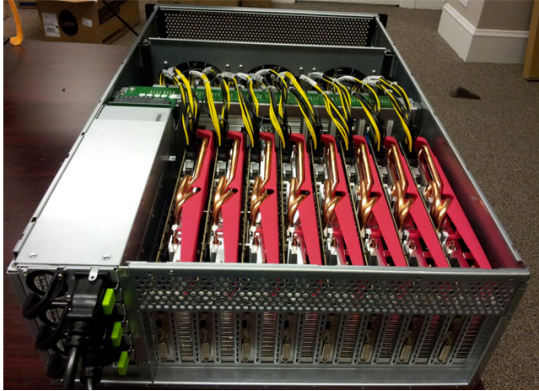
Welcome to Radeon City, population: 8. It's one of five servers that make up a high-performance password-cracking cluster.
